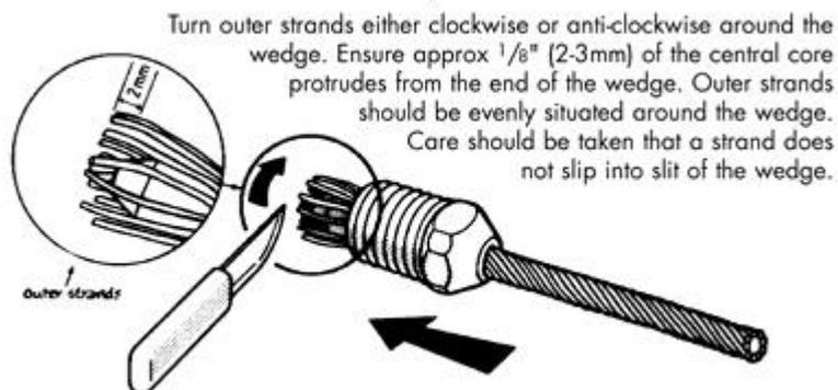
**TIP** Push the socket towards end of wire, while repositioning outer strands, this will help control. When wire strands are in position push socket firmly, as indicated to hold wires in position
