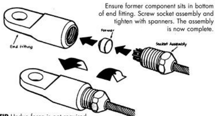
**TIP** Undue force is not required to terminate the wire.
